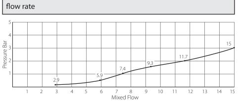
Flow rate curve is for reference only. The actual pressure drop may vary depending on system temperature and pressure.
