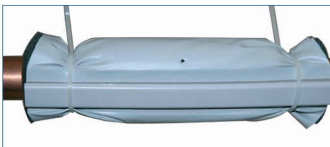
Fig. 1. Shows an Arctic Spray Freezing Jacket being attached to a pipe horizontally. Note the hole in the freezing jacket, this is where the Arctic Spray will be injected into the jacket. On horizontal freezes, use only the cable ties provided. There is no need to tape up the ends of the jacket.
