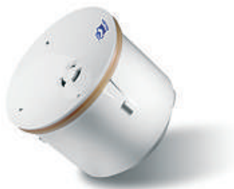
The Sealtrap cartridge - urine flows down the surface of the urinal and into the cartridge which is filled with a special liquid called Allseal. Foul air is prevented from rising up from the drain and into the washroom.
