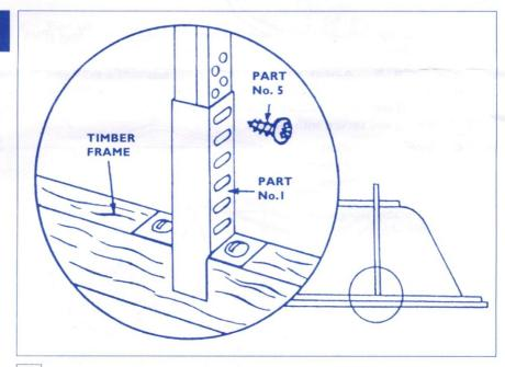
**a** Secure the sockets to the timber frame using the <sup>1</sup>/2" self tapping screws Part No. 5.
