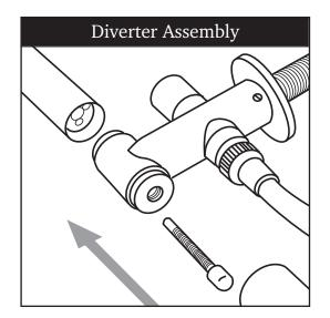
Remove backnut and washer from thread, push head through wall and connect to water supply. Secure with backnut and washer behind wall. Push diverter into bottom of pole, and secure with long brass screw. Screw the bottom tube into the bottom of diverter.
