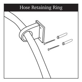
Push hose through the ring and secure to wall using screws and rawl plugs.
