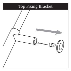
Screw flange and peg to wall using rawl plug. Push riser pole over peg and secure with grub screws.
