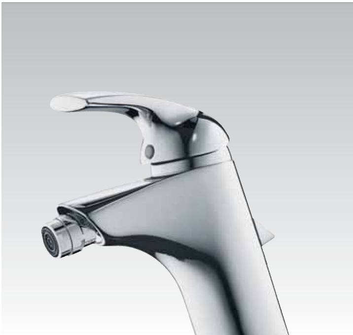
Tonic A5072 1 hole single lever bidet mixer 1/2" projection 128mm, pull knob pop-up waste 1 1/4" hot water limit stop, adjustable water saving device top fixation
